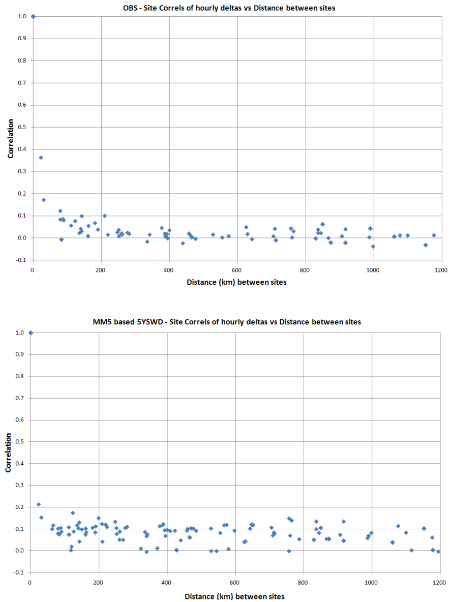
Figure 16: Correlations of hourly deltas between each of the 15 sites as a function of distance a) as observed (when possible), b) the MM5-based SWD.
