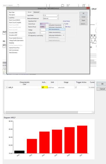
Alternatively, a script (DeleteLoadTrigger.ComDPL) is provided which disables all of the active load triggers.
