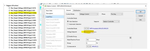
Note that the final voltage of the controlled bus may not be the value of the trigger because of the droop setting of the station controller – refer to the Station Controller Technical Reference for more details regarding droop (available through the PowerFactory help menu).
